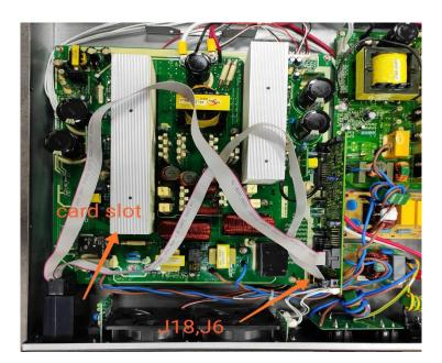
Please install SNMP card slot and connect signal cable to control board J18, J6.
