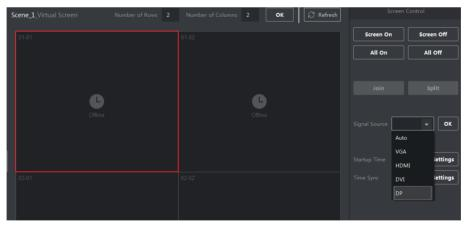
Figure 4-8 Switch Signal Sources by Drop-down List
