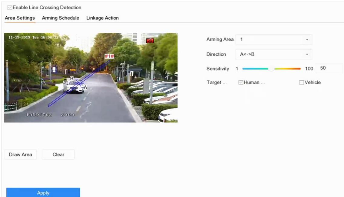
**Figure 7-12 Line Crossing Detection**
