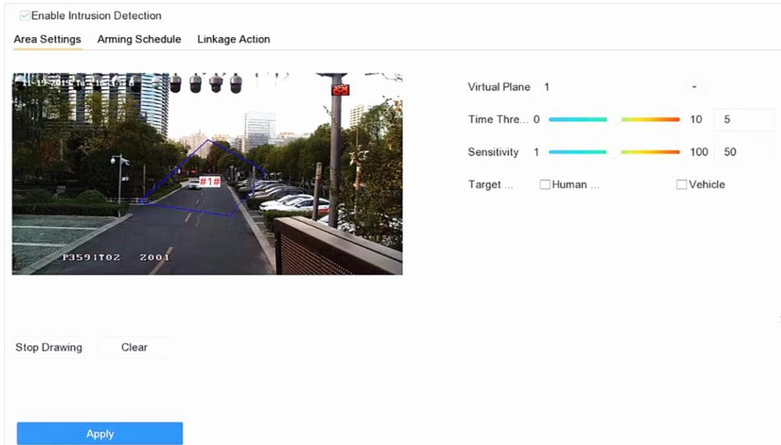
**Figure 7-13 Intrusion Detection**
