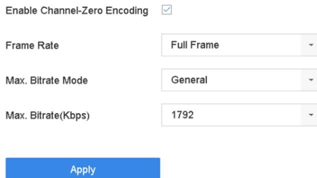
The screenshot shows a configuration interface for Channel-Zero Encoding. It includes a checked checkbox for 'Enable Channel-Zero Encoding', and three dropdown menus for 'Frame Rate' (set to 'Full Frame'), 'Max. Bitrate Mode' (set to 'General'), and 'Max. Bitrate(Kbps)' (set to '1792'). A blue 'Apply' button is located at the bottom.
