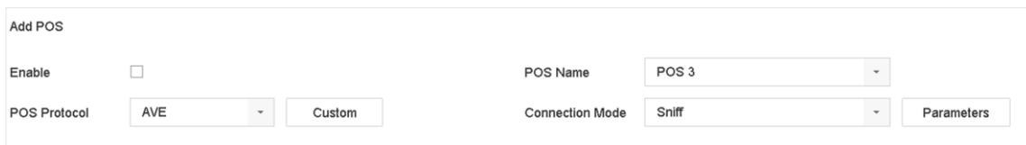
The screenshot shows the 'Add POS' configuration window. It includes an 'Enable' checkbox, a 'POS Name' dropdown menu with 'POS 3' selected, a 'POS Protocol' dropdown menu with 'AVE' selected and a 'Custom' button, and a 'Connection Mode' dropdown menu with 'Sniff' selected and a 'Parameters' button.
