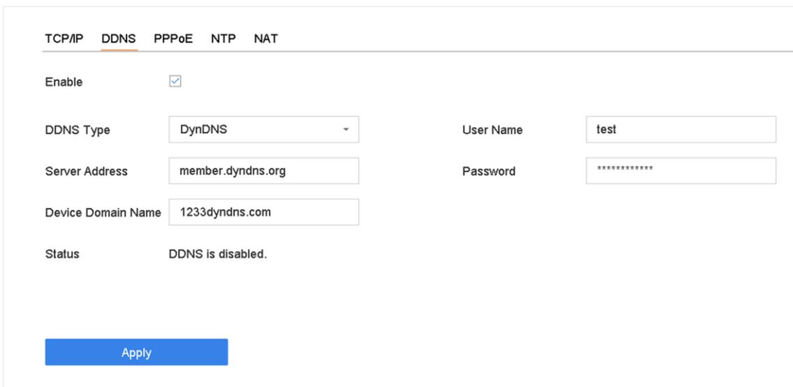
The screenshot shows the DDNS configuration page. At the top, there are tabs for TCP/IP, DDNS (selected), PPPoE, NTP, and NAT. Below the tabs, there is an 'Enable' checkbox which is checked. The 'DDNS Type' is set to 'DynDNS'. The 'Server Address' is 'member.dyndns.org'. The 'Device Domain Name' is '1233dyndns.com'. The 'User Name' is 'test' and the 'Password' is masked with asterisks. The 'Status' is 'DDNS is disabled.' and there is a blue 'Apply' button at the bottom.
