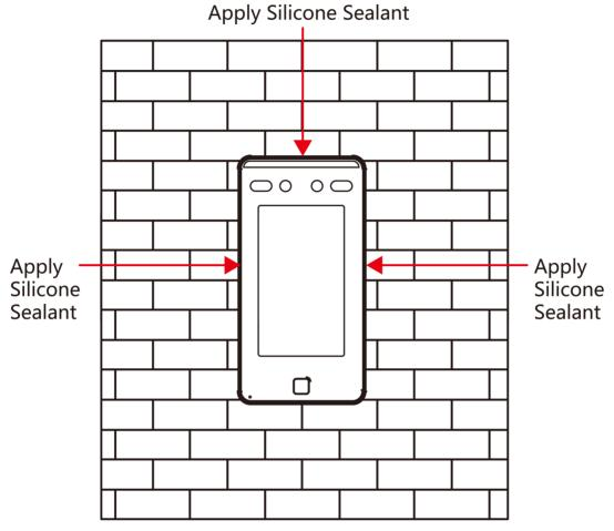
Figure 3-11 Apply Silicone Sealant on the Side
