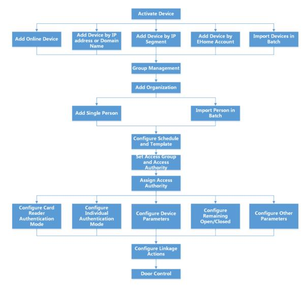
Figure 9-1 Flow Diagram of Configuration on Client Software
