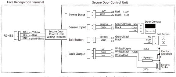
Figure 4-2 Secure Door Control Unit Wiring
