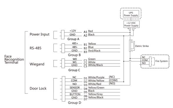
Figure 4-7 Device Wiring
