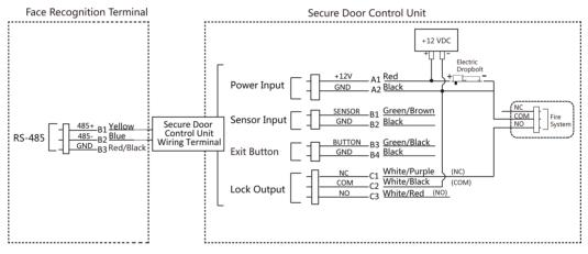
Figure 4-6 Wiring Secure Door Control Unit
