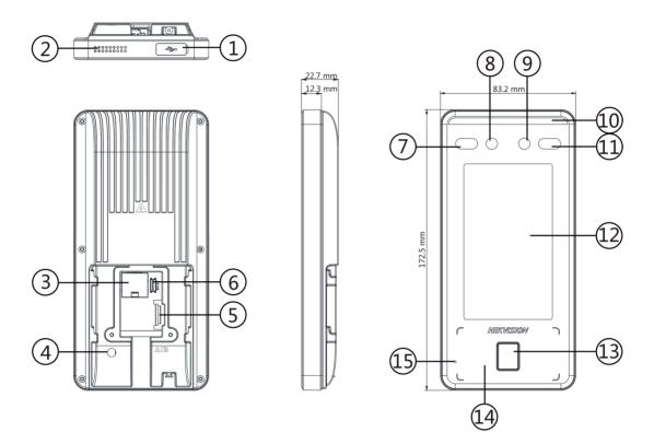
Figure 2-1 Face Recognition Terminal Diagram
