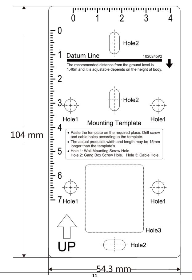
Figure 3-7 Mounting Template
