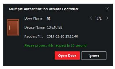
Figure 9-8 Remotely Open Door
