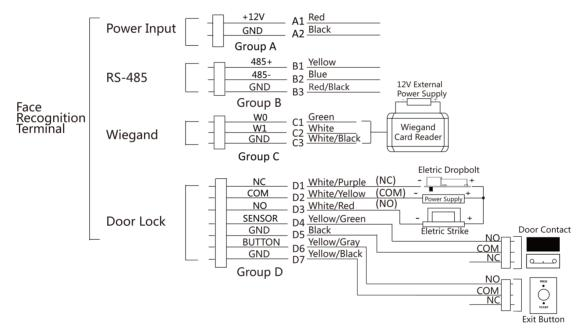
Figure 4-1 Device Wiring
