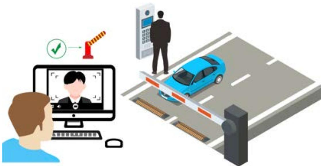
**Figure 18-8 Opening Barrier by Video Intercom**
