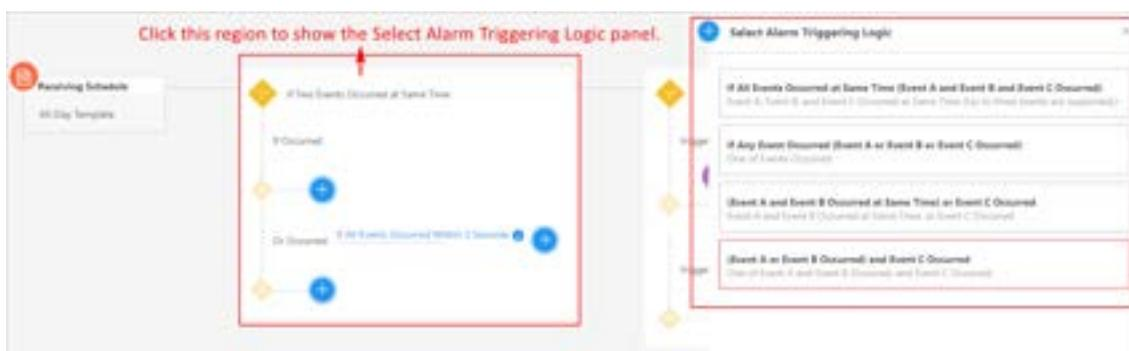
**Figure 13-10 Select Triggering Logic**
