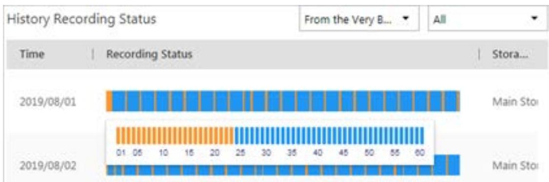
Figure 29-21 Recording Status Details within One Hour
