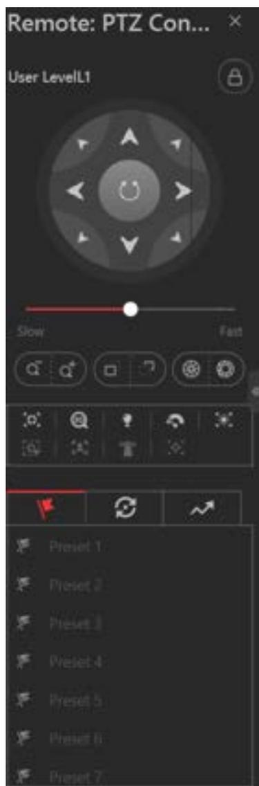
**Figure 14-8 PTZ Control Panel**
