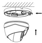
Figure 2-3 Secure the Camera
