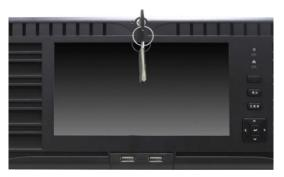
Figure 2. 2 Insert Panel Key
