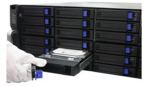
Figure 2. 10 Push the Hard Disk Box into the Slot
