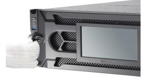
Figure 2. 12 Reinstall the Cover and Lock the Panel
