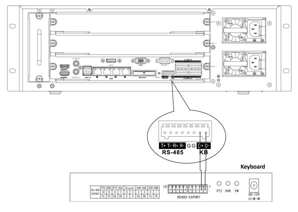
Figure 2. 15 Controller Connection
