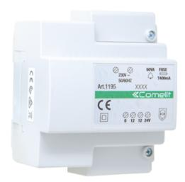
Transformer applicable to din rail (5 modules), input 230 VAC / 50÷60 Hz, output 12/24 VAC with terminal strip
